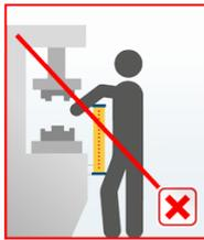
Fig. 7: Installation at a low safety distance
